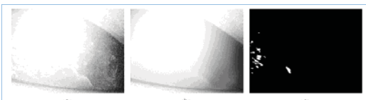
Figure 5. Image analysis for particle detection. (a) Original infrared image, (b) background estimation, (c) binary image with possible particles for velocity measurement.
